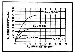
**Typical N-Channel Sink Current Characteristics**
