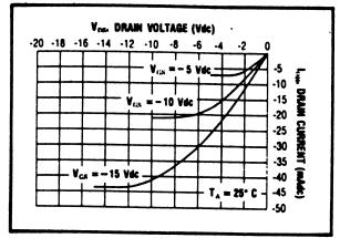
**Typical P-Channel Source Current Characteristics**
